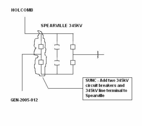
Figure 1. Interconnection Configuration
