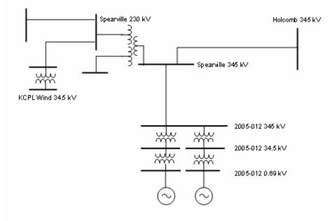
In addition to the base cases and interconnection configuration, the Customer provided the Project data consisting of generating units and their generating stepup transformers. In order to simplify the model of the wind farm, the wind turbines were aggregated in such a manner as to have one equivalent unit for several turbines connected to the same 34.5kV feeder end point.
